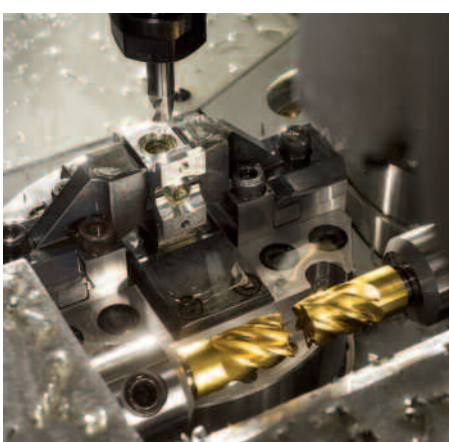
Combined machining: vertical and horizontal milling simultaneously with two tools
