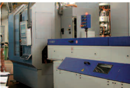
Mikron TB-600 enables bar loading with possibility of pre-machining (milling, turning)
