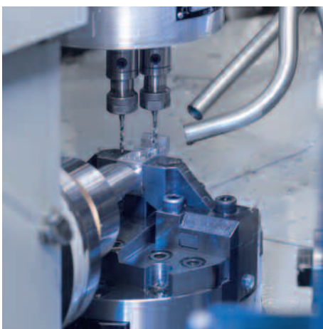
Machining with vertical multiple spindle
