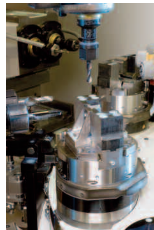
Combined machining: vertical and horizontal drilling with double spindle
