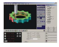
MeasureMind 3D provides complete control of touch probes for measuring features inaccessible by video or laser.
