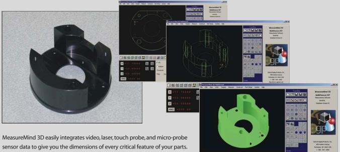
sensor data to give you the dimensions of every critical feature of your parts. Rich graphics and detailed numeric results help you relate measurements to design drawings. Rotate the part model to see hidden feature relationships. Rendered 3D models help you visualize the results, while tolerance variations appear in different colors. Tell at a glance which features are in or out of spec.
