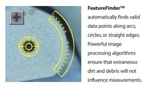
FeatureFinder™ automatically finds valid data points along arcs, circles, or straight edges. Powerful image processing algorithms ensure that extraneous dirt and debris will not
