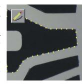
A trio of Weak Edge Point tools reliably and accurately find and measure extremely faint or indistinct edges. Weak Edge tools make it easy to find localized minimum or maximum points.
