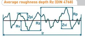
Average roughness depth Rz (µm) is the arithmetical mean of the individual roughness depths of five adjacent measuring sections,  $lr=1/5 \times (Z_1+Z_2+Z_3+Z_4+Z_5)$ .
