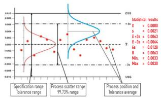
The machine capability index Cm and Cmk is calculated, subsequent to a machine capability analysis, using the following formula.
