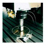
(grid and read head) Roundness test with measurement range Ø 140mm / Ø 230mm to Ø 2μm. Contactless optical measuring process, track speeds up to 80m/min, system accuracy 2 μm per axis, free form tests for testing any desired contours in two axes.
