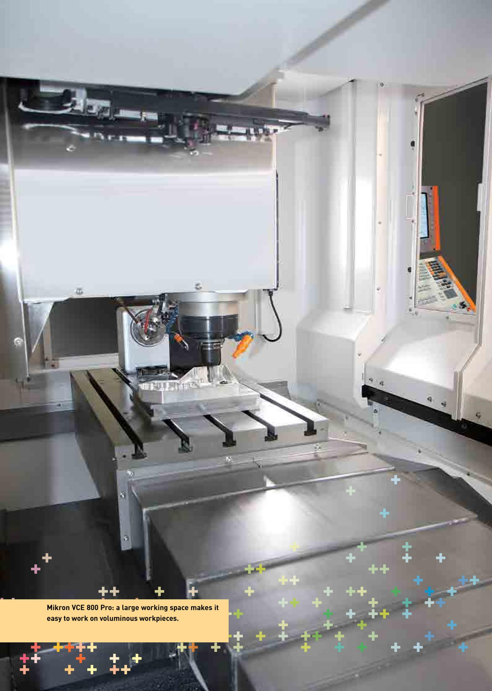
**Mikron VCE 800 Pro: a large working space makes it easy to work on voluminous workpieces.**
