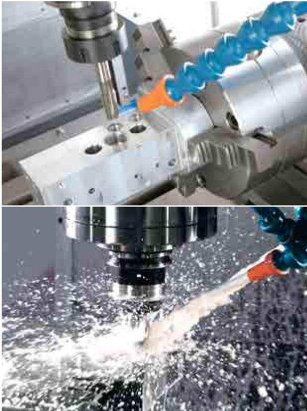
**Belt-driven spindle 6,000 rpm, 10,000 rpm, 14,000 rpm
