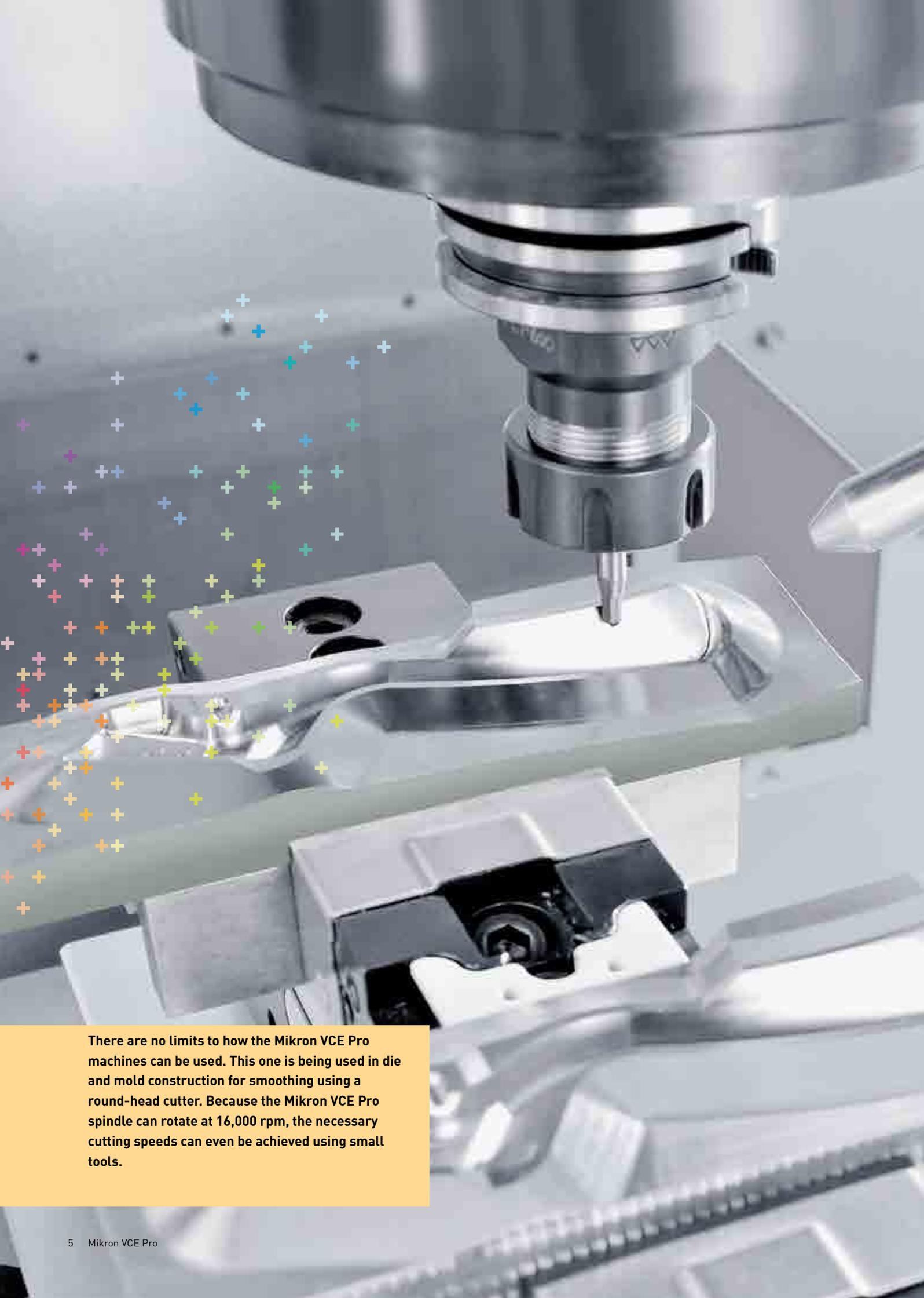
There are no limits to how the Mikron VCE Pro machines can be used. This one is being used in die and mold construction for smoothing using a round-head cutter. Because the Mikron VCE Pro spindle can rotate at 16,000 rpm, the necessary cutting speeds can even be achieved using small tools.
